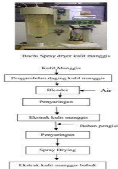
Figure 3.2 Grooves of Making Mangosteen Peel Extract into Powder
