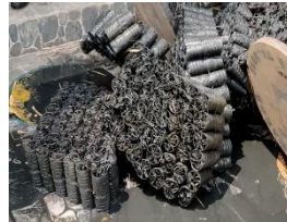
Figure 8. Existing Biofilter Media from Packaging Bottles
