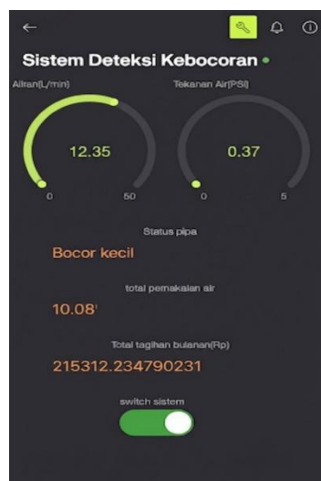
Figure 10. System detects small leakage anomalies
