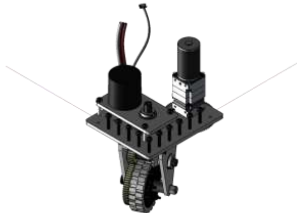
Figure 2. Design of a prototype of a swerve drive
