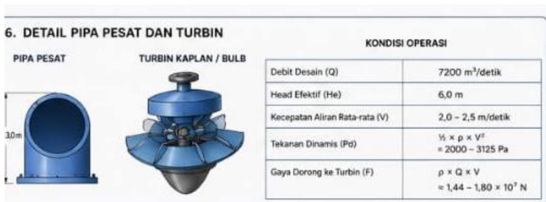
Figure 3. Detail of the penstock and Kaplan/Bulb turbine arrangement with the design operating conditions (Q, He, V, dynamic pressure Pd, and turbine thrust F).
