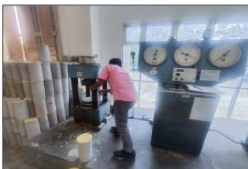
Figure 10. Compressive Strength Testing
