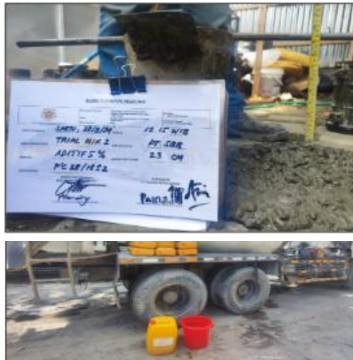
Figure 2. Addition Preparation Sikacrete-W dan Viscocrete-3115N
