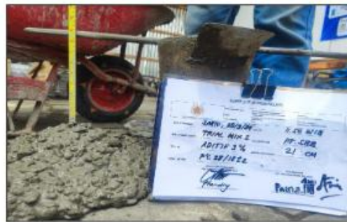
Figure 6. Slump Test on 3% mixture Sikacrete-W
