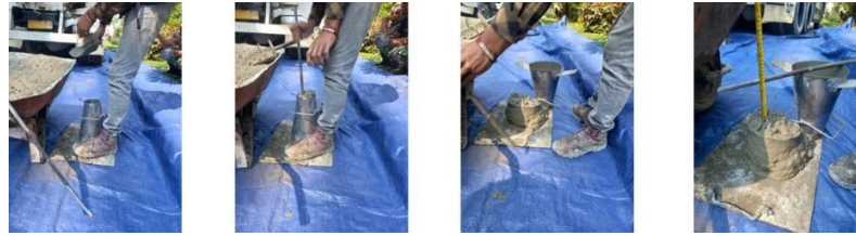
Figure 2. The Slump Test process in the field is at the Gatot Subroto Hospital Pump House Project in Central Jakarta with Contractor PT. Citra Nusa Padjadjaran
