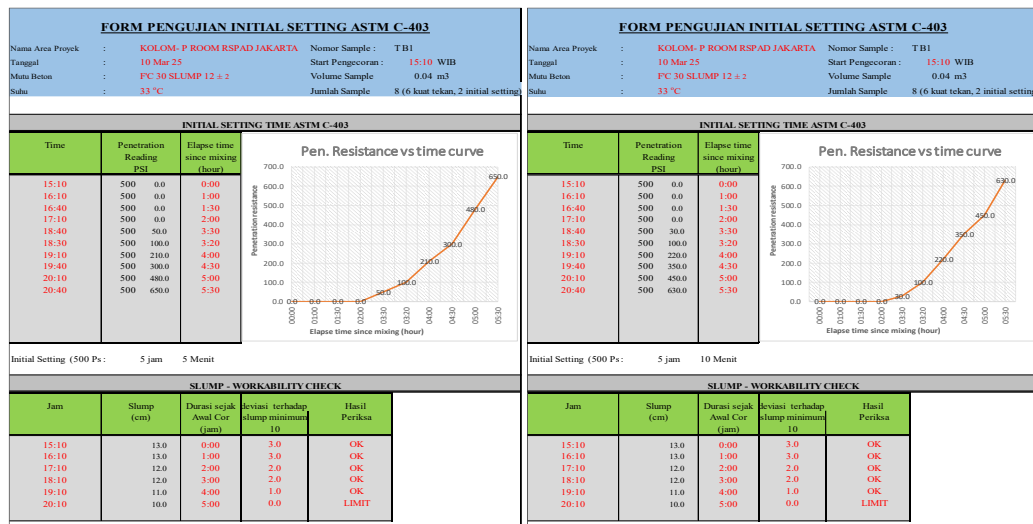
Figure 7. Initial setting test results on fresh concrete with additive content of 0.3%
