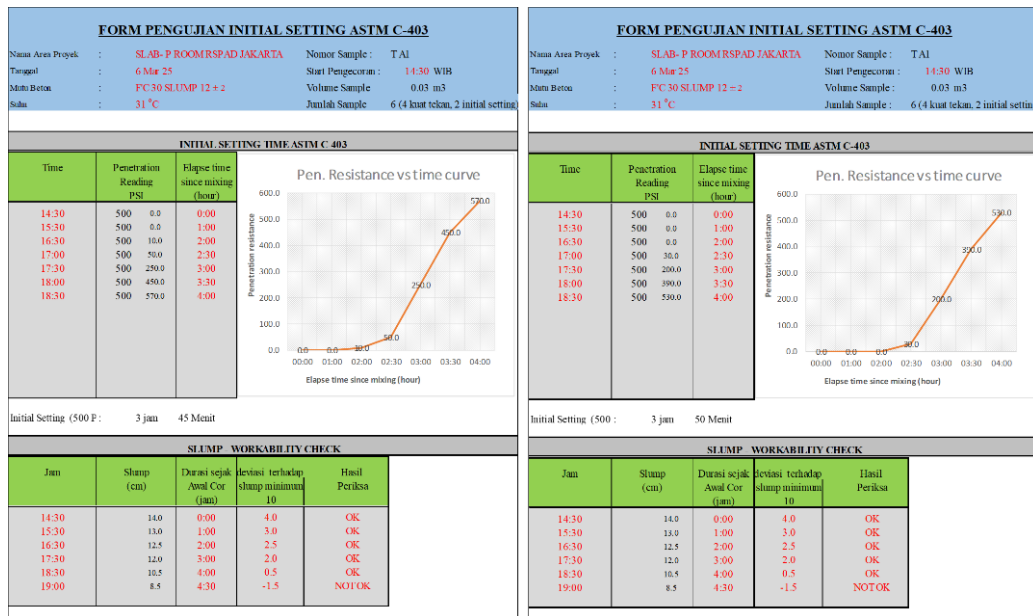
Figure 6. Initial setting test results on fresh concrete with additive content of 0.2%
