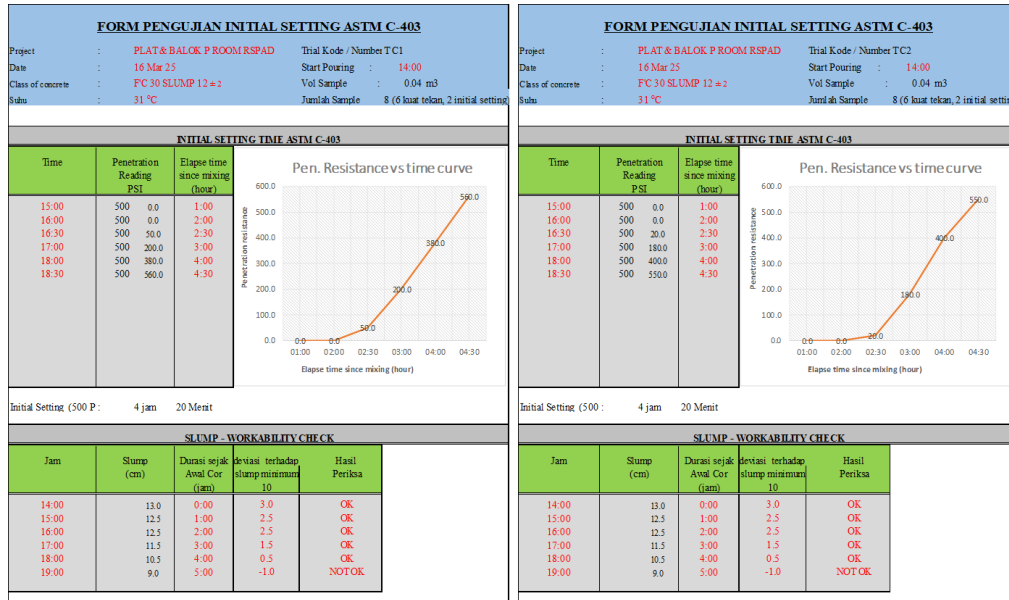
Figure 8. Initial setting test results on fresh concrete with additive content of 0.25%
