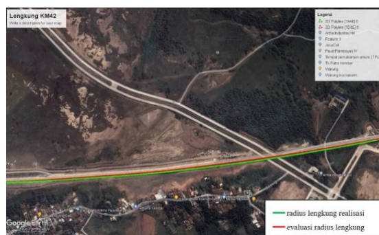
Figure 5. Horizontal arch evaluation KM 42+410
